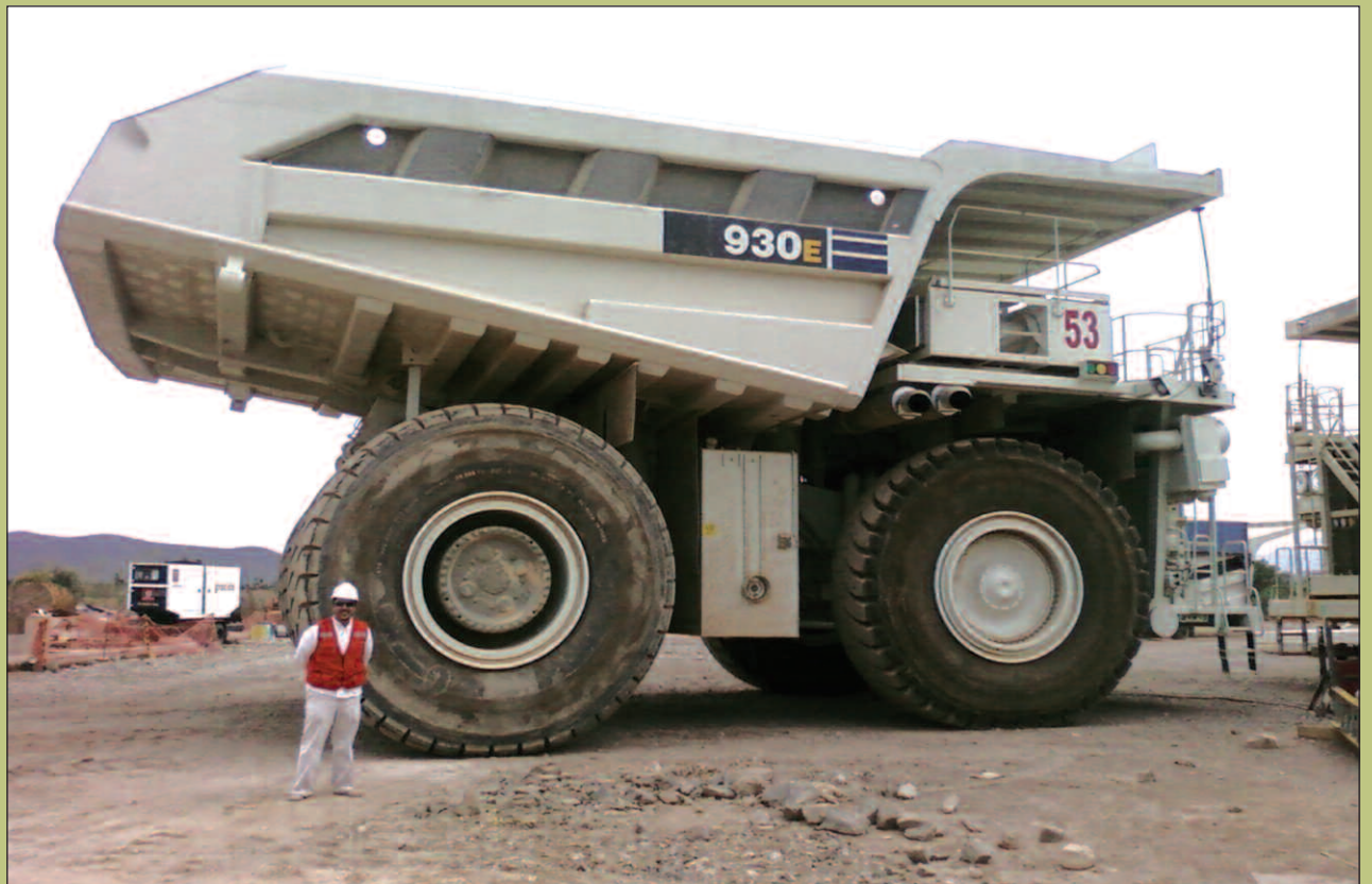
This haul truck carries over 200 tonnes
